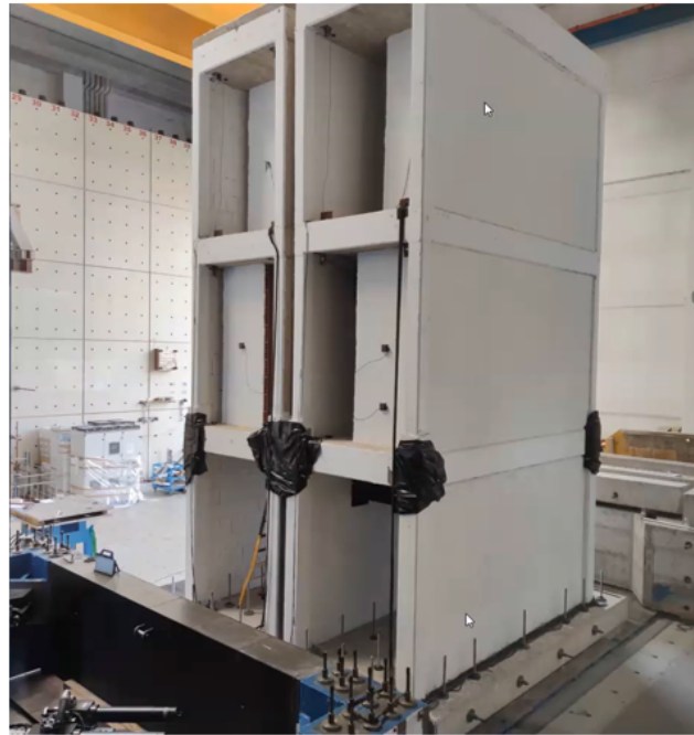
Figure 3.2: Twin full-scale RC buildings mounted on the unidirectional shaking table. Building 1 (left) is as-built; Building 2 (right) is retrofitted.
