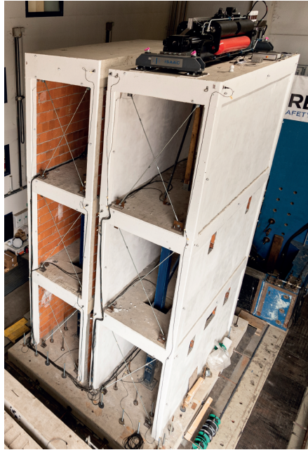
Figure 3.3: View of the two RC buildings on the shaking table with the internal steel safety frame in the central bay. The frame is bolted to the foundation slab and to the slab of the third floor and is used as a safety device during the shaking-table tests.
