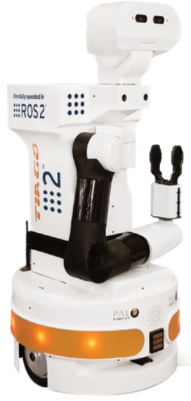
Figure 3.1: Model of the PAL Robotics TIAGo one-arm platform used for the project
