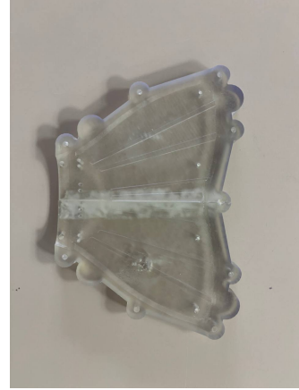
(b) Fin after printing and cleaning
