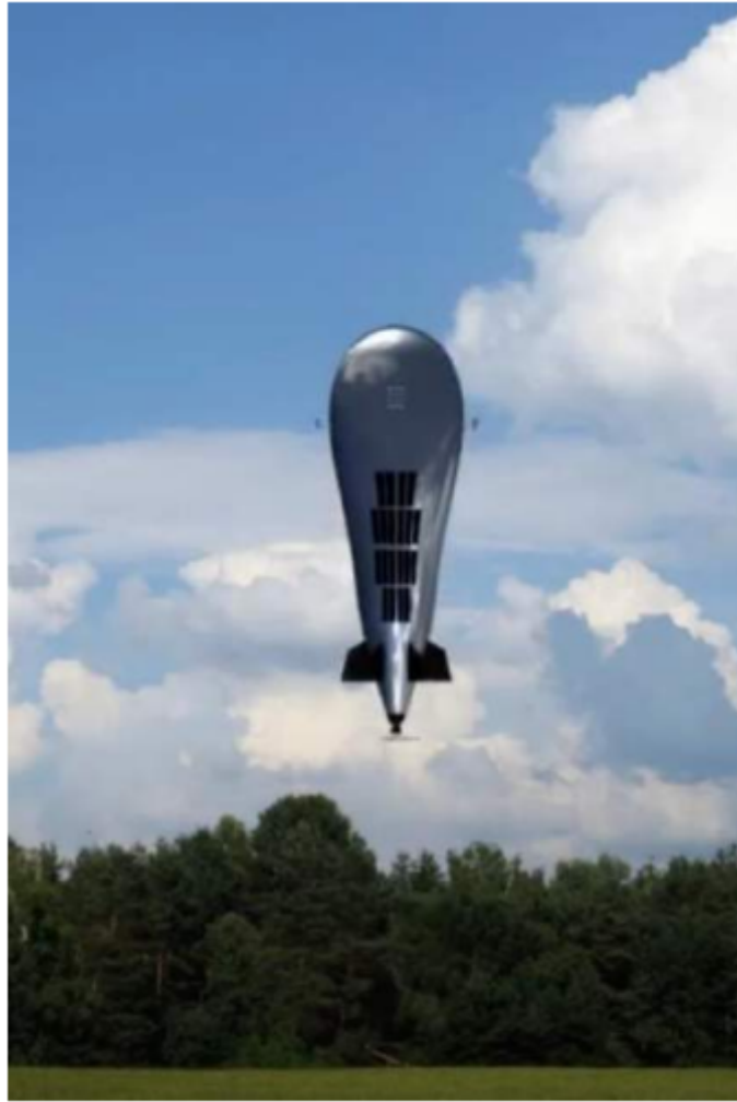
Figure 2.4: Vertical launch configuration of the HHAA (partially inflated) (courtesy: CIRA) [1].
