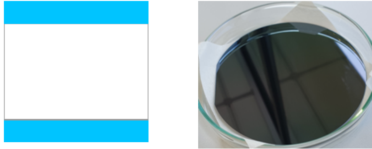
Figure 3.2: Initial 1 mm Si + 2 \mu\text{m} \text{SiO}_2 wafer
