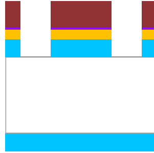
Figure 3.9: SiO 2 etching step
