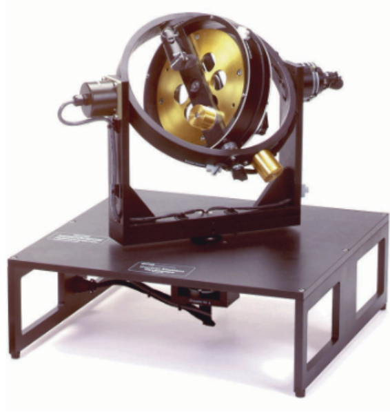
Figure 4.2. Dual Gimbal Variable Speed Control Moment Gyro.
