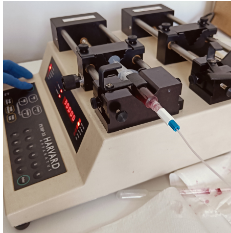
Figure 2.26: Syringe setup used for microfluidic leakage tests, with Syringe Pump model 33 from Harvard Apparatus [17] .
