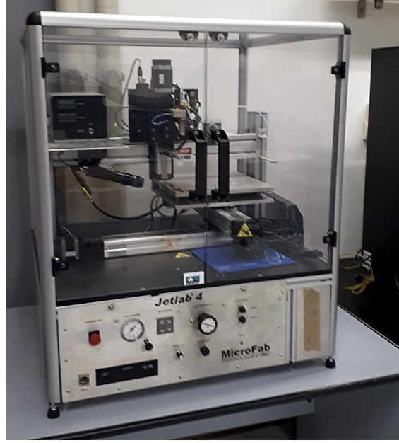
Figure 2.21: Jetlab 4 DOD by MicroFab Technologies Inc. [13] , [14]
