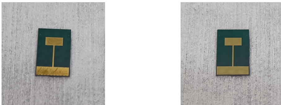
(a) Gate electrode after fabrication process, (b) Gate electrode after cleaning in acetone before cleaning. and isopropyl alcohol.
