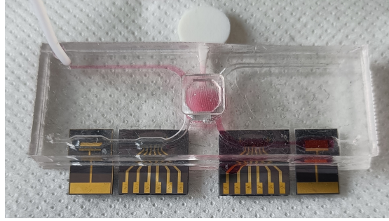
Figure 3.9: Microfluidic test showing the separation of the two channels by the Oxyphen membrane.
