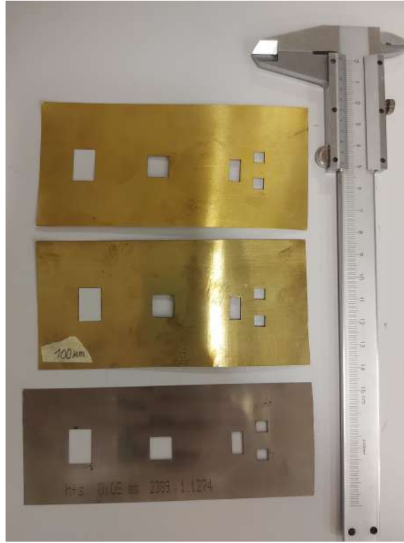
Figure 10.6: Metallic stencils, from top to bottom: brass 150 \mu m, brass 100 \mu m and steel 50 \mu m.
