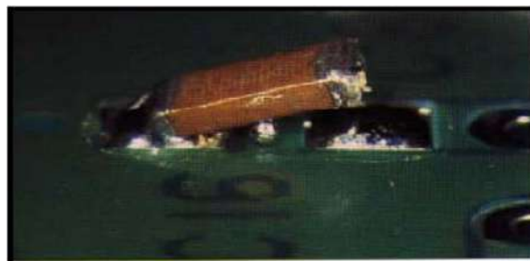
Figure 9.1: Tombstoning image[50] where the component is lifted similarly to a drawbridge.
