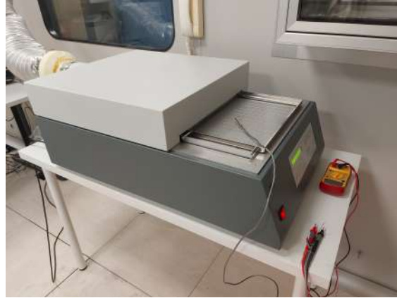
(b) MR10A oven and Thermoresistor/multimeter setup for temperature measurements.
