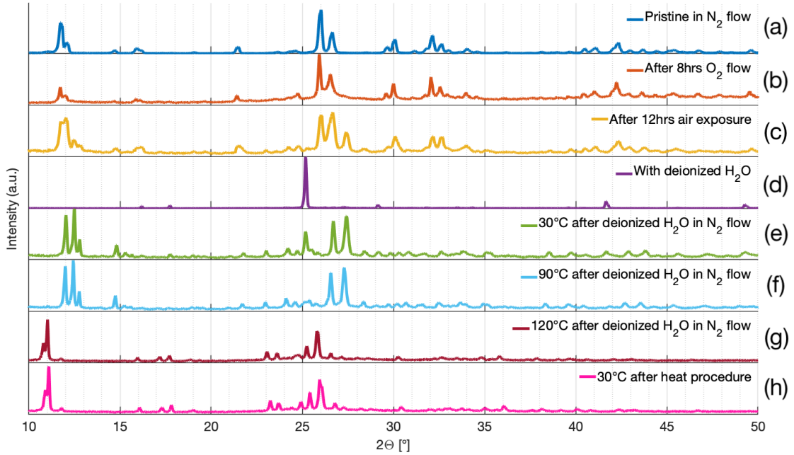
Figure 3.5: XRD patterns (acquired at @IIT-CCT, Genoa) of the most relevant phases observed during in-situ measurements of \text{DMASnI}_3 powder. Chronologically, the patterns are shown top to bottom, starting from the pristine condition (a), oxygen only exposure (b), ambient air exposure (c), de-ionized water (d). Panels (e),(f),(g) and (h) instead represent a summary of a longer heat experimental test conducted after water exposure. Each pattern is discussed in detail later on.
