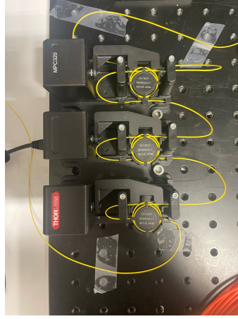
Figure 3.6: Photo of the Thorlabs motorized polarization controller (MPC320) utilized in this work.
