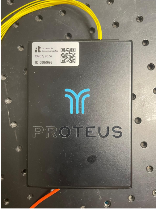
(a) MPLC device (Cailabs, model PROS_10_0002_1550) used during the experimental characterization.
