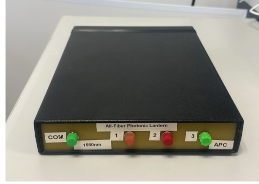
(b) PL device used in this thesis, featuring 1 FMF input and 3 SMF outputs.
