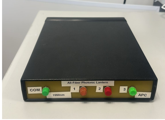
Figure 2.3: Photograph of the PL device used in this thesis, featuring 1 FMF input and 3 SMF outputs.
