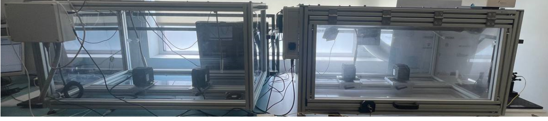
Figure 4.1: In this experiment the FSO link is composed of two fiber collimators, separated by two atmospheric chambers.
