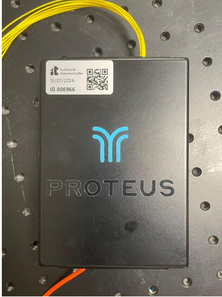
Figure 2.5: Photograph of the MPLC device (Proteus, Cailabs) used in this thesis, featuring 1 FMF input and 10 SMF outputs.
