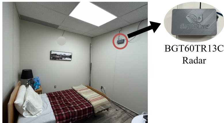
Figure 3.7: Bedroom layout and radar placement in the home-like data collection environment.
