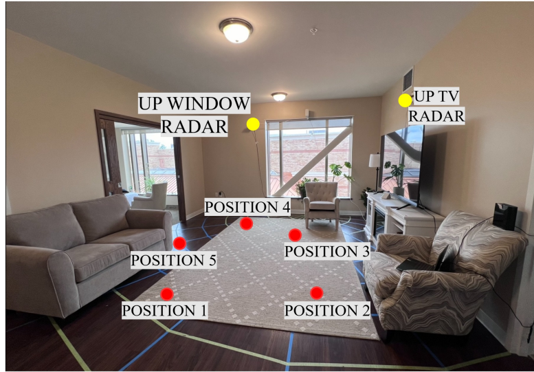
Figure 3.13: The living room layout indicating radars positions and activity locations.
