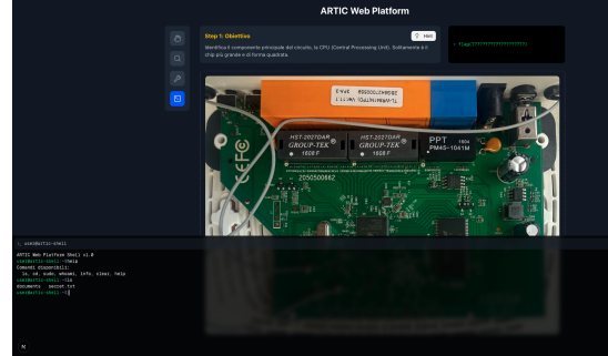
Figure 4.2. Interactive Serial Access: Once pins are identified, a virtual terminal console opens, replaying our complete bootlogs and responding to bootloader or shell commands based on recorded behavioral models.
