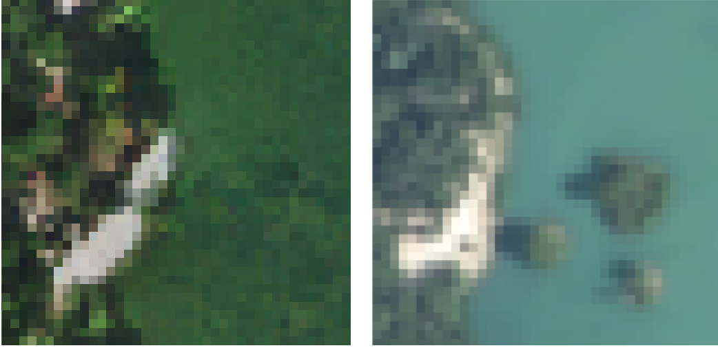
Figure 5.1. Example of the output produced by the pre-trained ESRGAN model, with the super-resolved image on the left and the HR target on the right. The model tends to overestimate the presence of green areas and vegetation, while excelling at reconstructing fine details and textures (e.g., trees).
