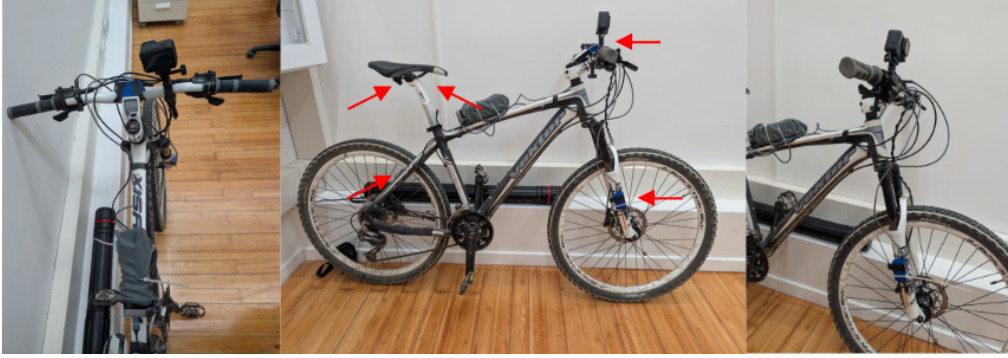
Figure 3.15: Bicycle with mounted sensors, used in the road-surface detection use case
