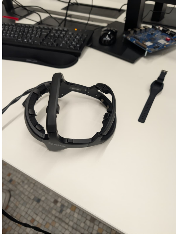
Figure 3.18: Sensors used for third case study: EEG headset and Metawear wearable bracelet
