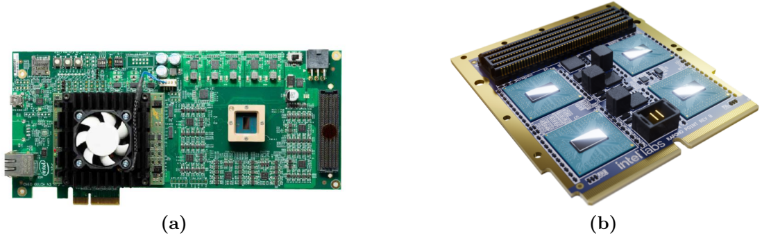
Figure 2.5: Two of the available Loihi 2 hardware: Oheo Gulch on the left and Kapoho Point on the left.
