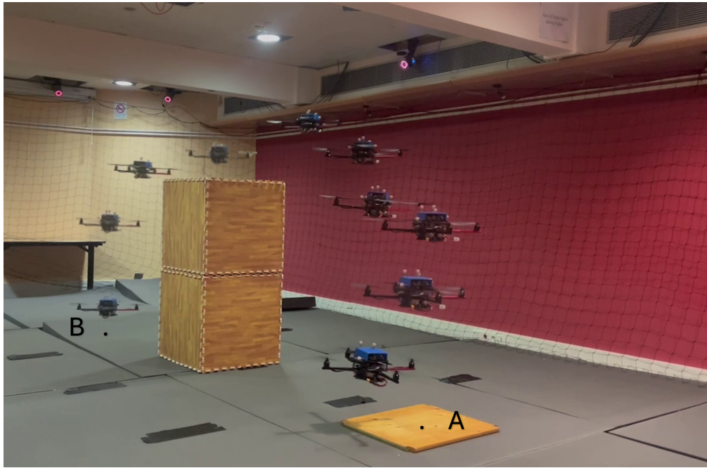
Figure 4.22: Multi-exposure photograph showing overlaid drone positions during avoidance maneuver. Point A marks start, structure B represents target point, and frame sequence illustrates lateral deviation trajectory.
