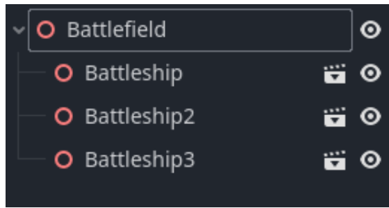
Figure 3.1: An example of a scene (the battlefield) containing multiple instances of the same Battleship scene. The red circle represents the Node3D node, which is usually used as a root node for a 3D scene. Adding another battleship is as easy as dragging the scene into the battlefield one.
