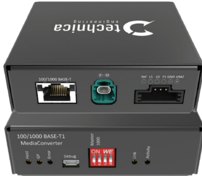
Figure 4.2: Cable connectors for the 100BASE-T1 side are chosen to be HMTD, compliant to most automotive network solutions. Source: [8]
