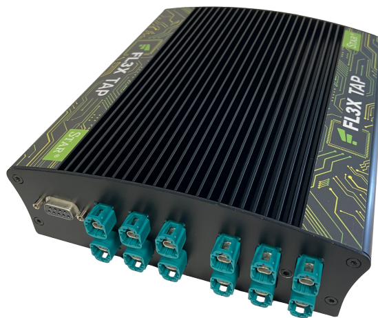
Figure 4.4: Cable connectors for input data stream are HMTD type. Front LEDs assure the link establishment and data flowing through the PHYs and the logging ports. Source: [10]
