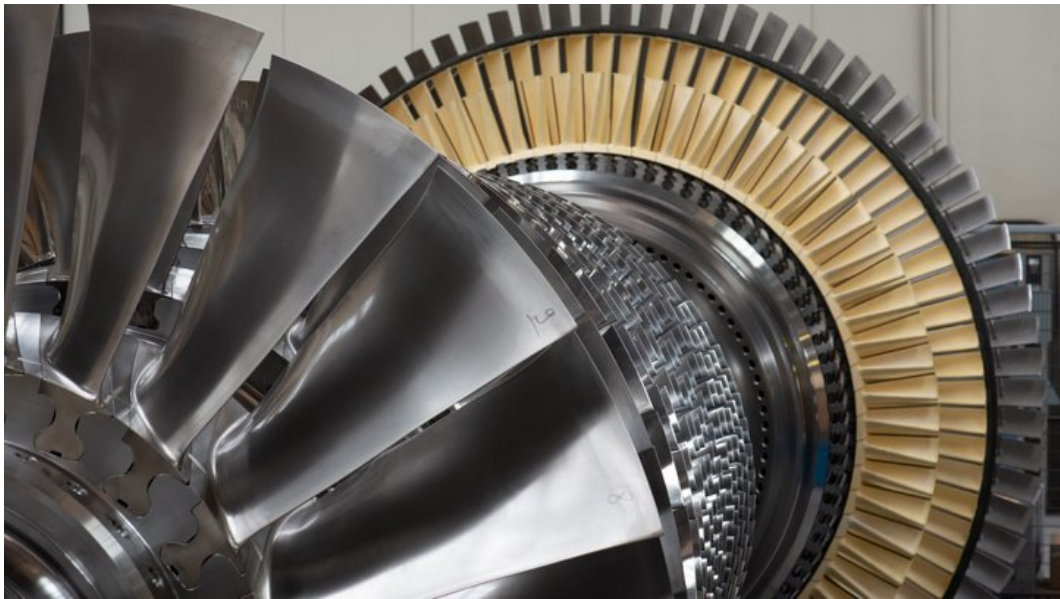
Figure 1.4: Compressor Stage during Assembly process [1]
