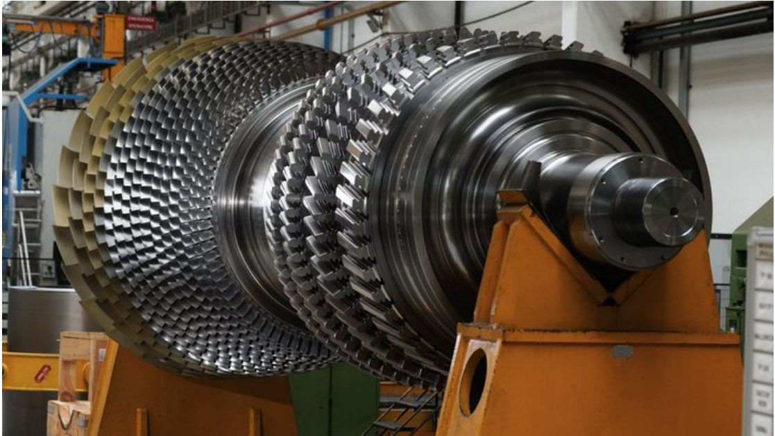
Figure 1.5: The Rotor during the assembly process [1]
