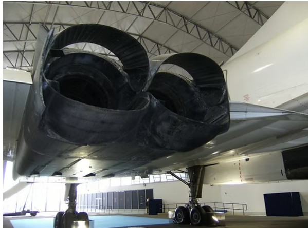
Figure 5.17: Concorde exhaust nozzle [23]
