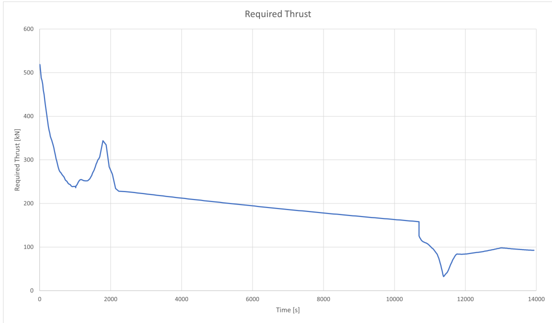
Figure 7.3: Required Thrust for Concorde (four engines)
