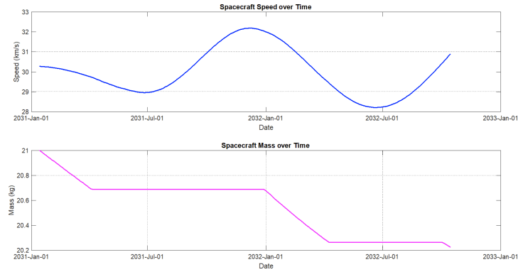
Figure 5.3: Mass consumption during the mission and its effect on the spacecraft's heliocentric speed
