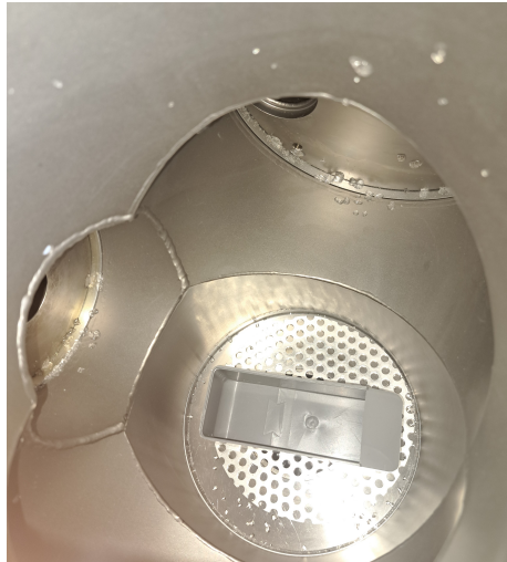
Figure 7.14: Naphthalene condensation inside the chamber
