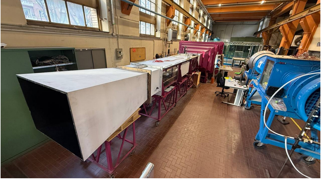
Figure 2.1: boundary layer wind tunnel of Laboratory of Aeronautics M. Panetti of Politecnico di Torino.
