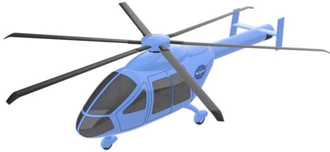
Figure 2.14: Schematic of a quiet single-main rotor helicopter configuration (adapted from Johnson [21]).
