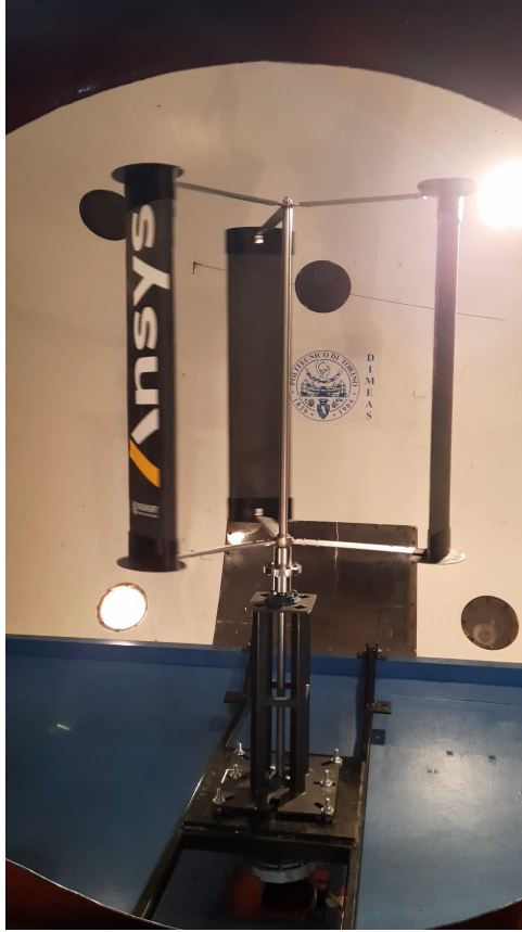
(a) Turbine as installed in the test section
