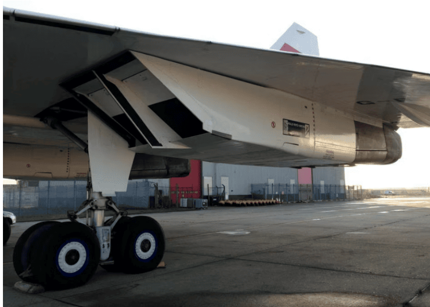
Figure 3.6: Concorde - Engine nacelles [22]
