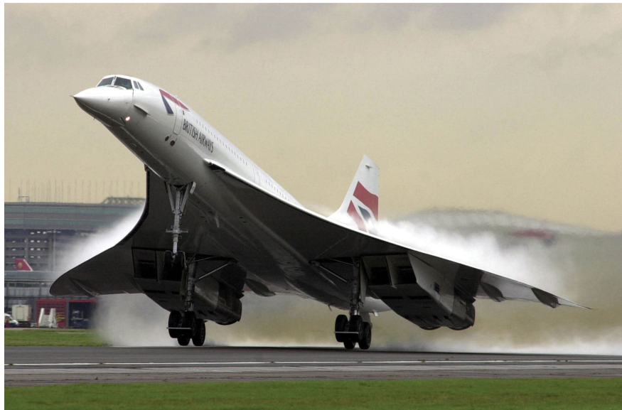
Figure 3.4: Phenomenon of vortex lift [22]
