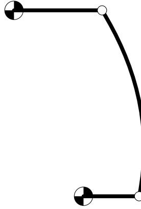
Figure 5.1: Sketch of the desired PACOMA leg after pretension.
