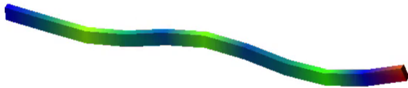
Figure 3.12: Representation of the fourth frequency: 6659.7 Hz
