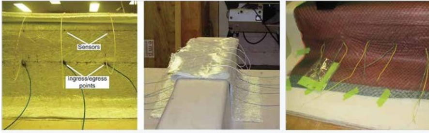
Figure 4.8: Material with Optical Fibres ready for infusion [42].
