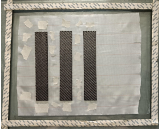
Figure 5.7: Optical fibre fixed on the peel-ply.
