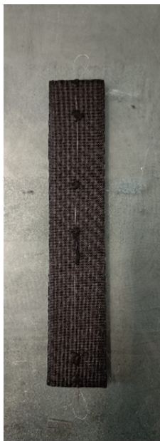
Figure 5.14: Specimen with fibre folded before the cutting.
