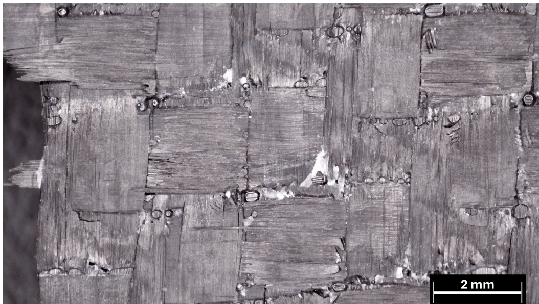
Figure 7.36: Enlargement of the fracture surface with small voids consistent with resin-rich pockets.
