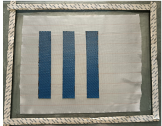
Figure 5.6: Prepreg strips laying on the peel-ply.
