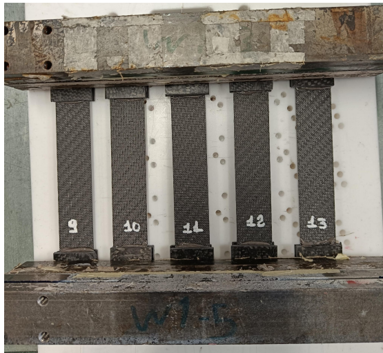
Figure 5.16: Specimens with tabs and weight applied.
