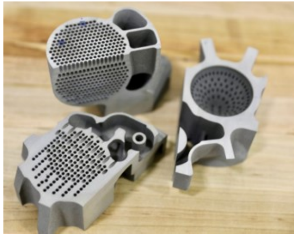
Figure 5.5: Cross-section of Additive Manufactured Production Heat Exchanger [12]
