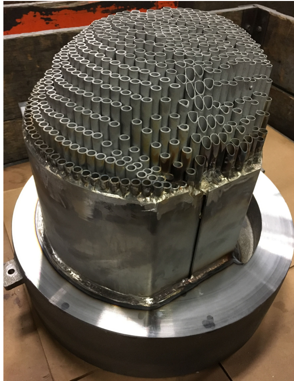
Figure 5.13: Emerson's conventionally produced anticavitation device involved many parts and skilled labor. Difficult and costly to produce [33]
