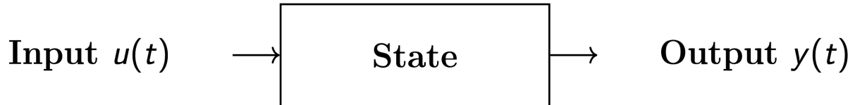
Figure 3.12: Conceptual representation of a dynamic system showing the input–state–output relation used for SysML–Simulink mapping.
