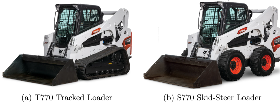
Figure 2.17: Examples of two identically sized Skid-Steer Loaders from Bobcat: Tracked and Wheeled. Source: Doosan Bobcat
