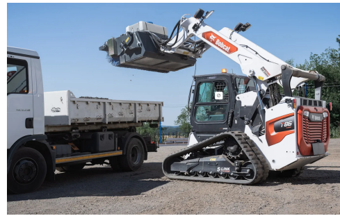
(b) Tracked Loader performing bucket emptying part of the duty cycle. Source: Doosan Bobcat
