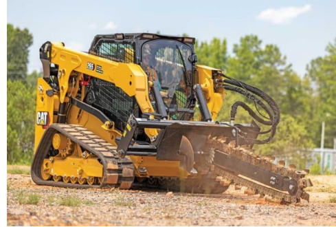
(b) Tracked Loader with a chain trencher attachment
