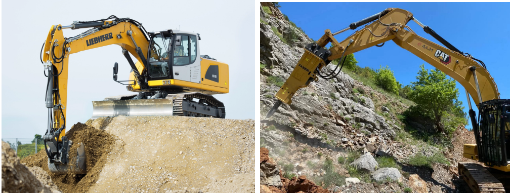
(a) Liebherr generation 8 crawler excavator in earthmoving application. Source: Liebherr [23]. (b) Caterpillar crawler excavator with hydraulic hammer attachment. Source: Fiore Ricambi ShPK
