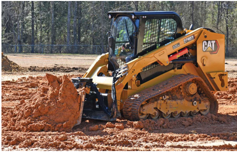
(a) Tracked Loader performing bucket filling part of the duty cycle. Source: Caterpillar Inc.
