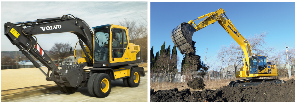
(a) Volvo EW145B Prime wheeled excavator. Source: Volvo Construction Equipment [24]. (b) Komatsu PC240LC/NLC-11 crawler excavator. Source: Komatsu [25].
