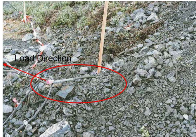
Figure 27: Bent solid bar anchor, due to shear, after impact (Ingram & Wagner, 2012)
