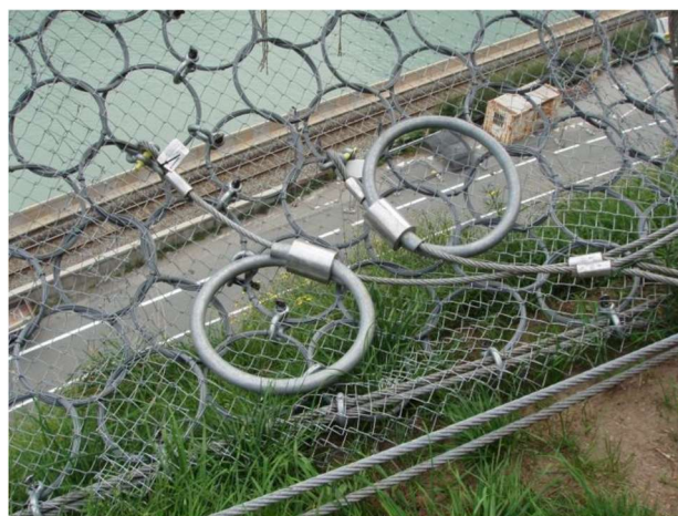
Figure 40: Mixed friction/plastic deformation ring brake system (Geobruigg, s.d.) (Marchelli M. , 2020)
