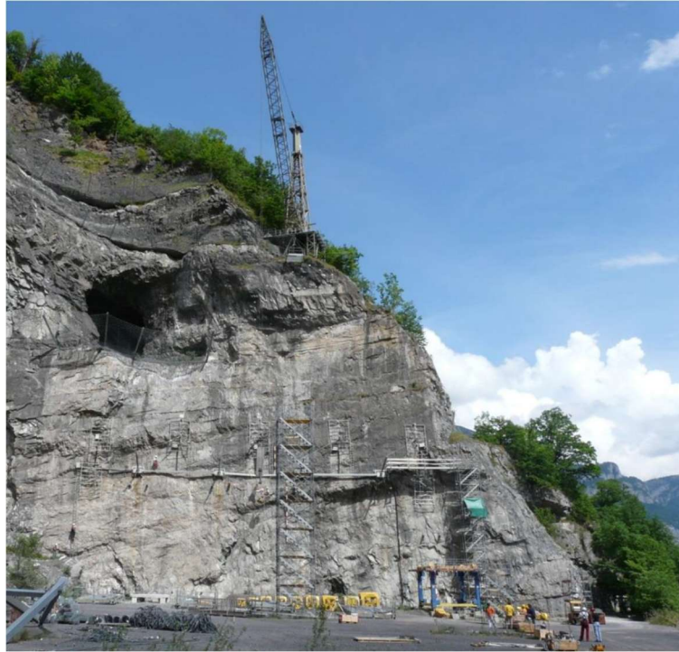
Figure 58: Walenstadt vertical drop impact test instrumentation and configuration (Marchelli M. , 2020)
