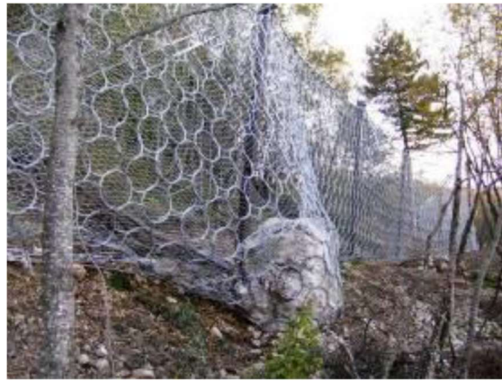
Figure 57: intercepted block in safe condition for real scale test (Marchelli M. , 2020)
