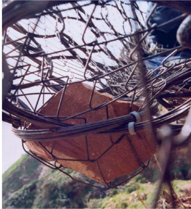
Figure 66: High-speed rockfalls can create high energies with quite small blocks and could puncture protection barriers loading smaller impact areas (Volkwein, Roth, Gerber, & Aron, 2009)
