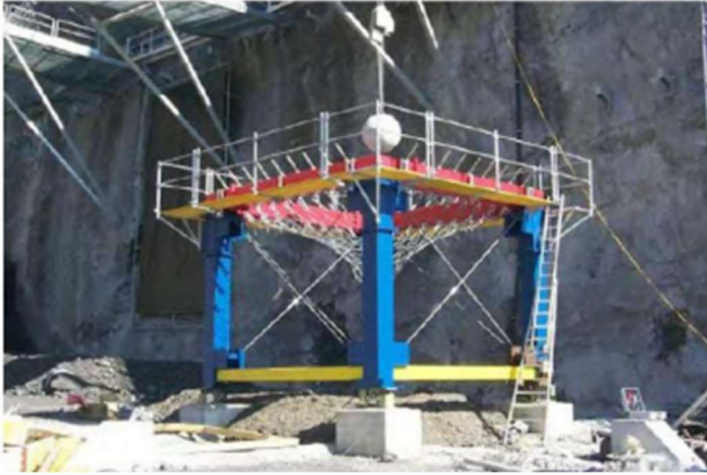
Figure 68: The specifically built Test Rig for Rockfall Tests, Front View (Koo & J.S.H., 2014)
