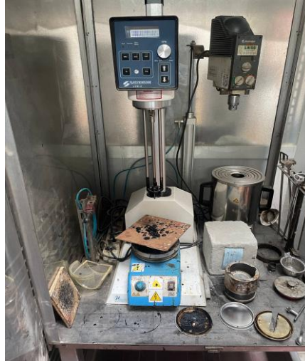
Figure 2.1.1.1 - High-Shear Mixer: Operated up to 5000 RPM by Silverson model L5M-A
