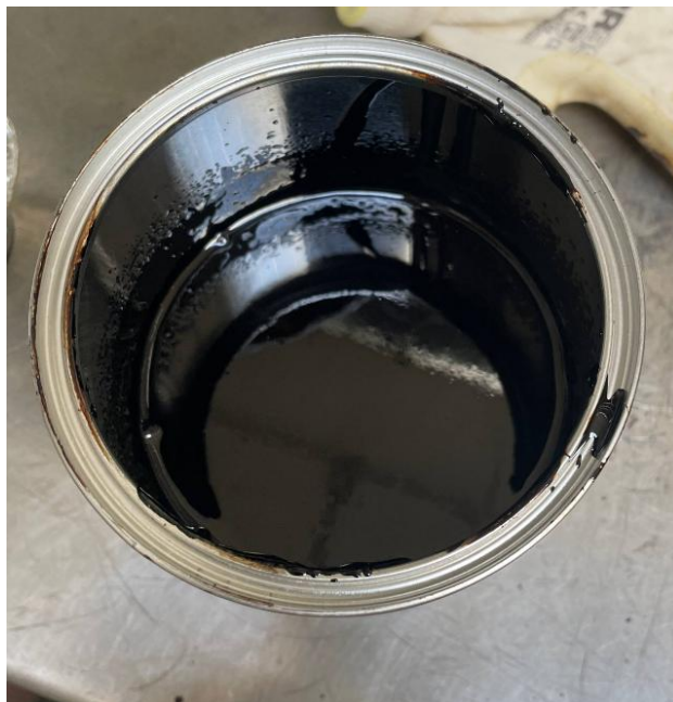
Figure 2.2.1 – Mixed binder with RLD-plastic.
