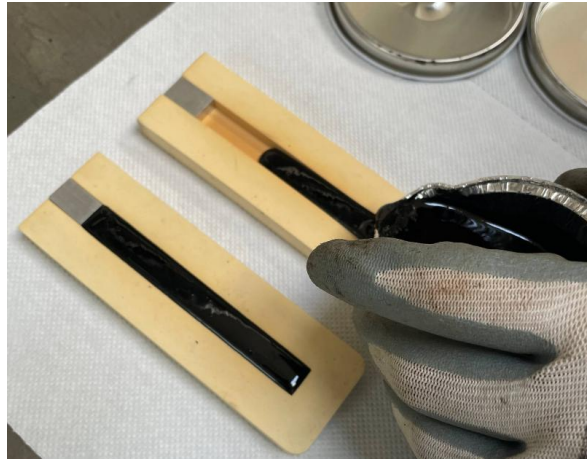
Figure 2.2.2 - Preparation of bituminous beams.
