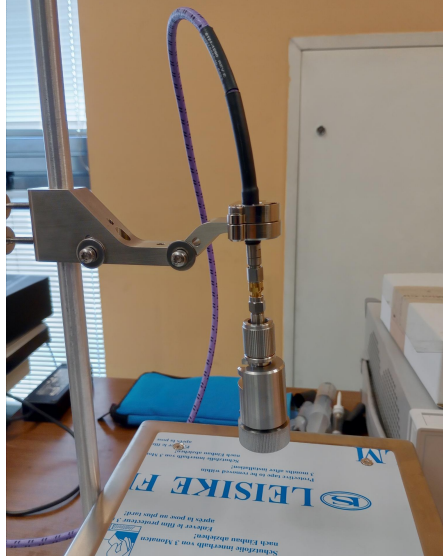
Figure 69: Dielectric probe setup for measuring relative permittivity and conductivity of filling materials
