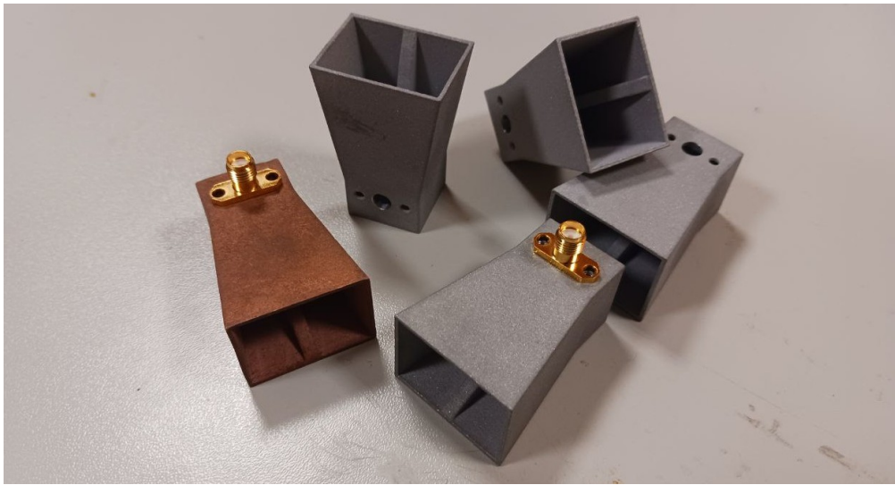
Figure 66: Fabricated antenna prototypes in aluminum and copper for microwave testing
