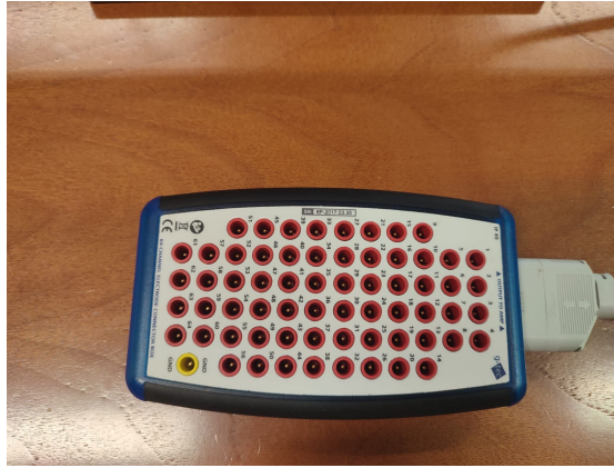
Figure 3.4: Frontal view of the gHIAMP connector box. The yellow input is dedicated to the ground connection.
