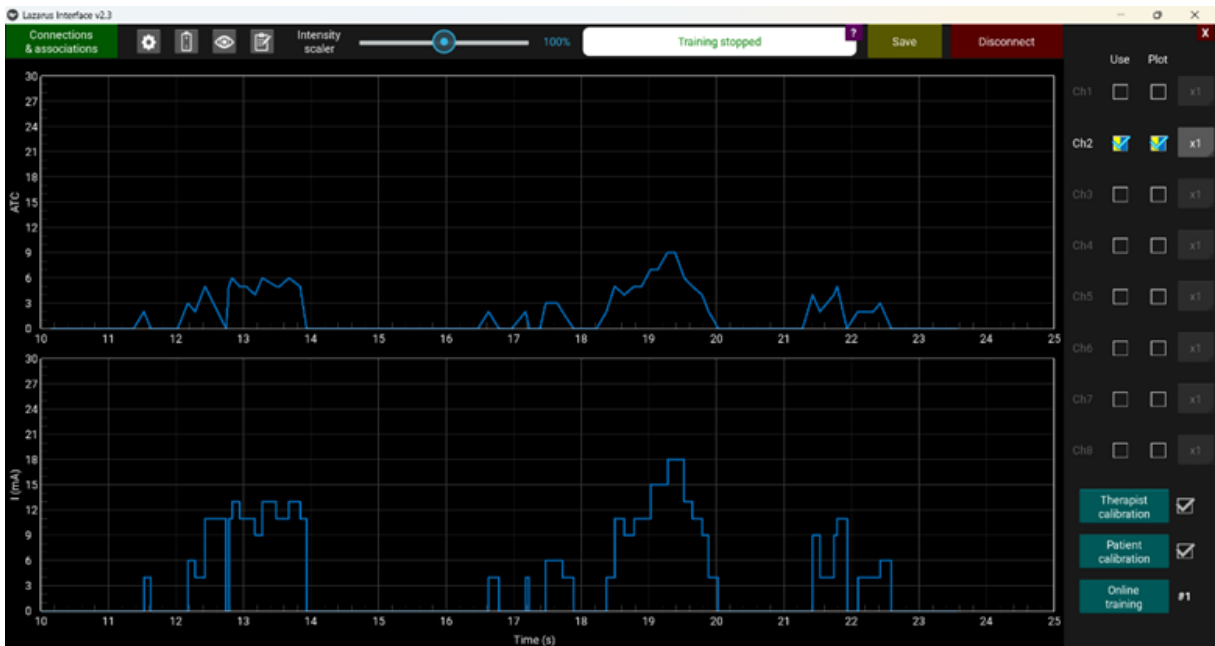
Figure 3.16: Example of the rehabilitation interface displaying, in real time, the ATC signal from the target muscle and the stimulation current delivered to the patient's arm.
