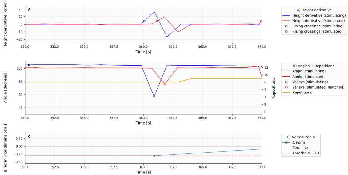
Figure 5.4: The program identifies the (a) start of the repetition from the height derivative, computes the (b) minimum angles of the stimulating and stimulated limbs, and verifies (c) that their normalized difference remains within the tolerance threshold.
