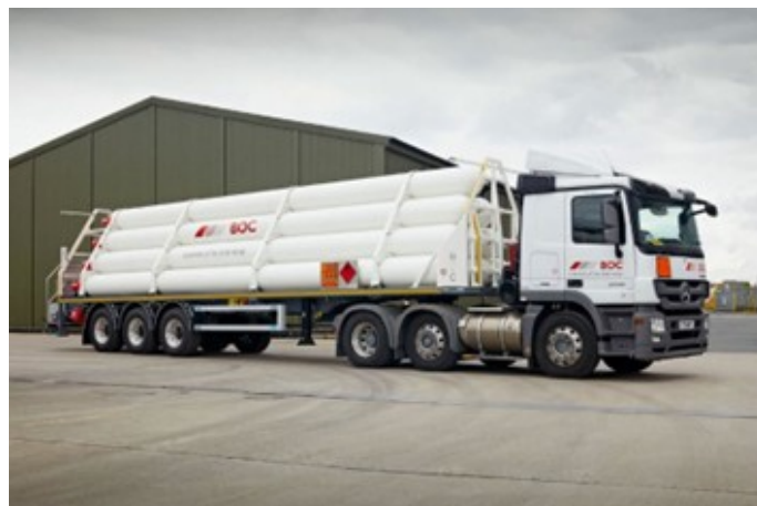
Figure 2.14: Tube trailer for transporting hydrogen [57]
