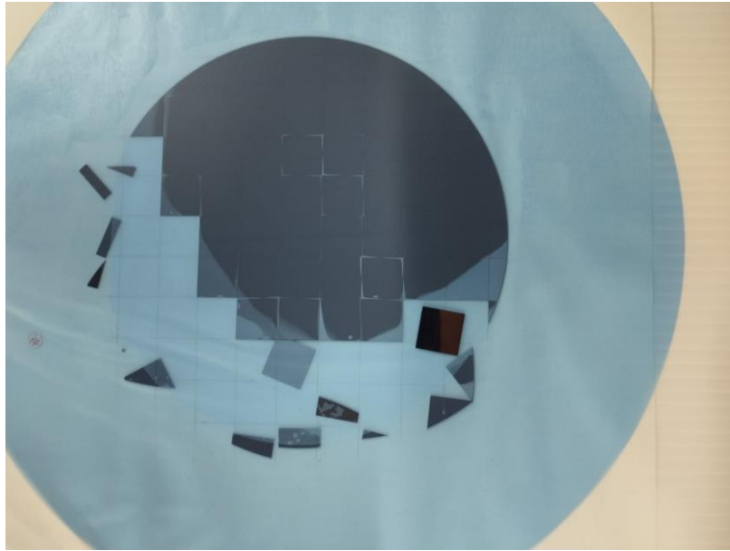
Figure 10: Silicon wafer cut and prepared for use ( 15 \times 15 mm squares)
