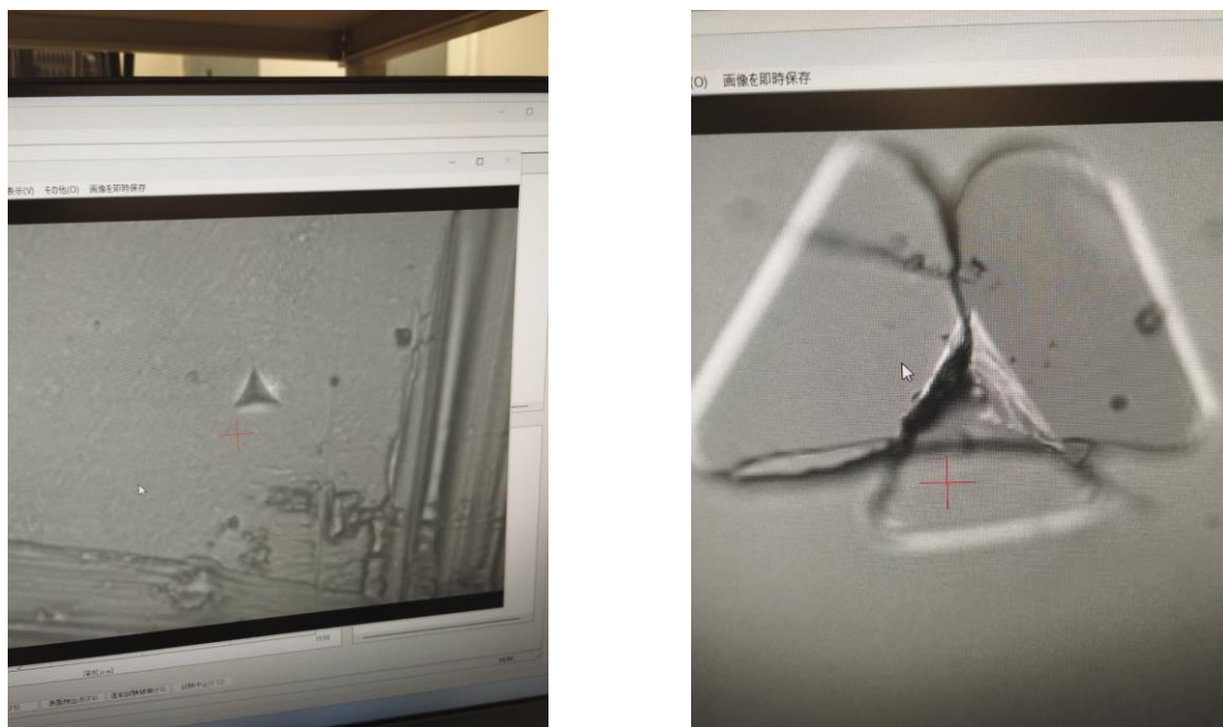
Figure 7: example of indentation with different force applied (1 \mu\text{m} scale bar).
