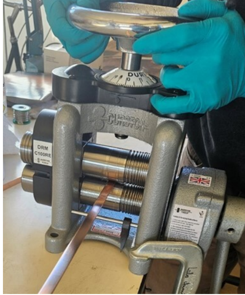
Figure 3.5: Rolling mill used to flatten 2 mm thick copper plates. The applied pressure must be low enough to correct the initial curvature without significantly altering the final plate thickness.
