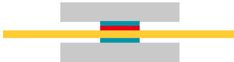
Figure 7.4: Setup for compression tests. Grey: press plates. Red: 5 cm copper plate. Yellow: conductor under test. Blue: teflon.
