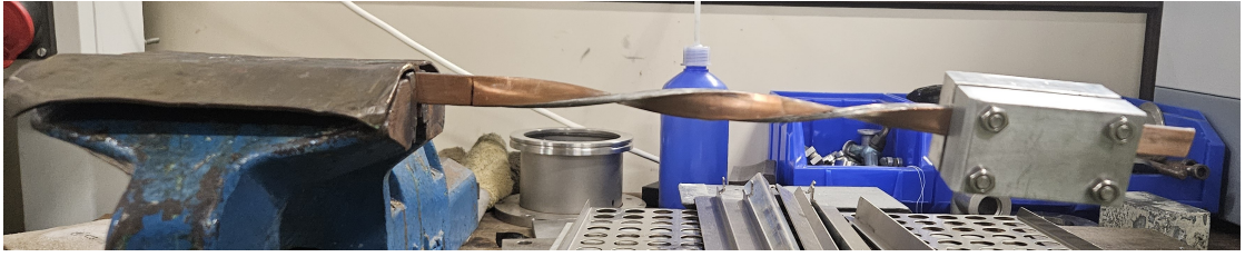
Figure 9.3: Conductor after applying a 360^\circ on a 20cm long section.
