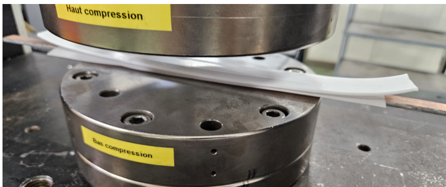
Figure 7.2: Compression test setup with Teflon sheets on both sides.
