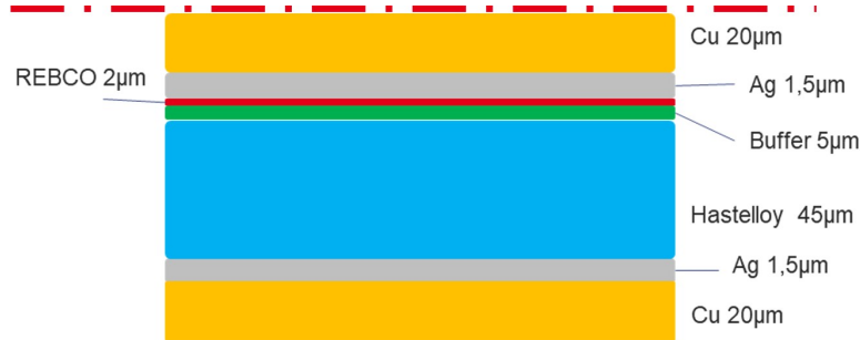
Figure 8.1: Schematic representation of the REBCO layers within the SST tape. The dashed line at the top represents the geometric center of the conductor. The REBCO layer is highlighted in red.
