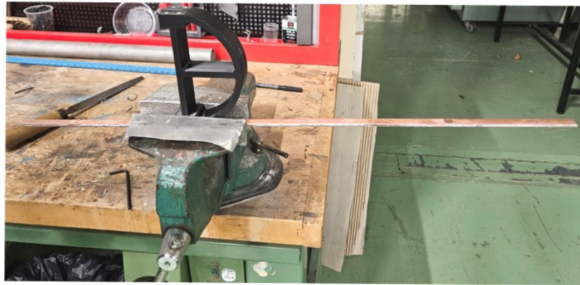
Figure 8.2: Process to achieve bending of the conductor. One end is clamped in a bench vise while the other is manually bent to adhere to the 3D-printed piece (in black).
