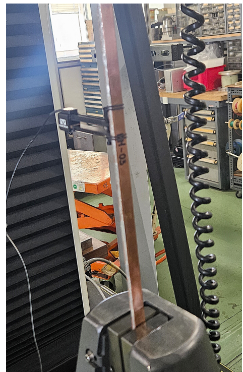
(b) Side view with extensometer
