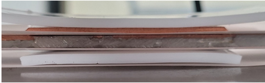
Figure 7.6: Side view of stacked elements. Prescale film was inserted between all layers to detect stress variations.
