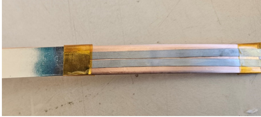
Figure 3.6: End section of the conductor during alignment. The grey area on the left shows the HTS tape, ending just before the copper plate (at the bottom). The two thin Sn63Pb37 strips, obtained from the rolling mill, are also visible. All components are held in place with adhesive tape.
