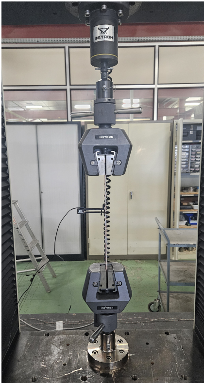
(a) Full front view of the tensile press
