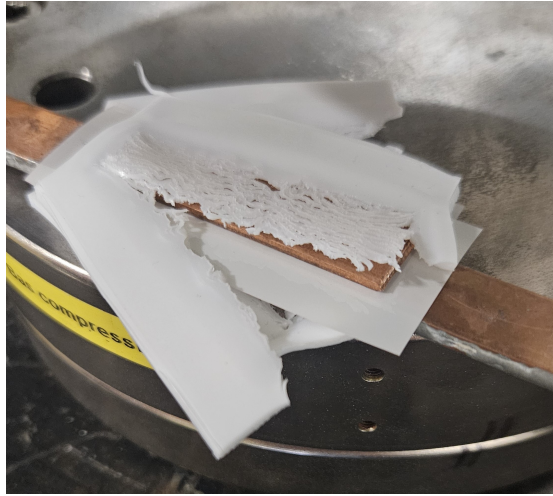
Figure 7.9: Rupture of the Teflon sheet following the 200 MPa compression test.
