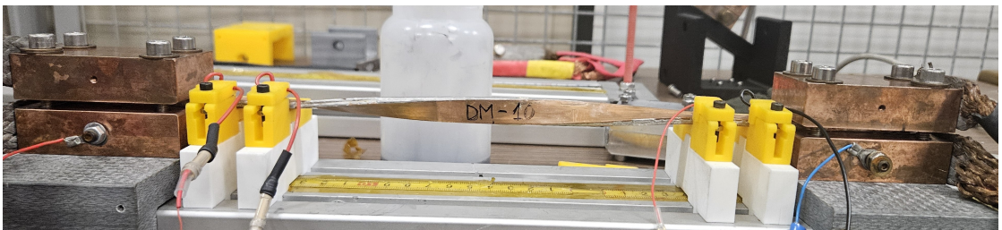
Figure 9.5: Front view of the test bench setup with the conductor positioned between the copper blocks for potential lead placement ( 180^\circ torsion on a 20cm long section).
