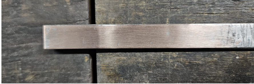
(b) DM-01 conductor after surface cleaning with abrasive cloth.
