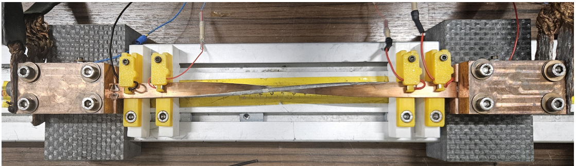
Figure 9.4: Top view of the test bench setup showing the conductor fixed between the copper blocks ( 180^\circ torsion on a 20cm long section).
