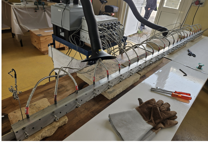
Figure 3.8: Setup used for assembling the 3-meter-long conductor, consisting of three heated presses connected in series.
