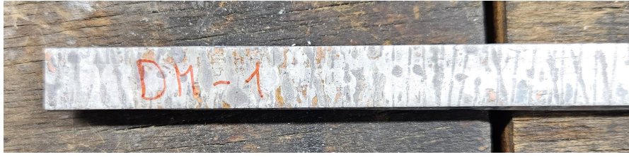
(a) DM-01 conductor before surface cleaning. Since it was assembled using method 1, the deposited SnPb layer also had to be removed.
