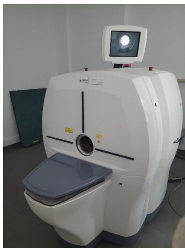
Figure 2.18: FLEX® Triumph® II preclinical imaging system (Gamma Medica) used for \mu SPECT/CT acquisitions.
