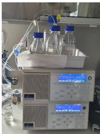
Figure 2.14: PerkinElmer Series 200 analytical HPLC system equipped with a UV-vis detector (Series 200 UV/VIS Detector) and a Supelco Discovery BIO Wide Pore C18 column (250 × 4.6 mm, 300 Å, 5 µm).
