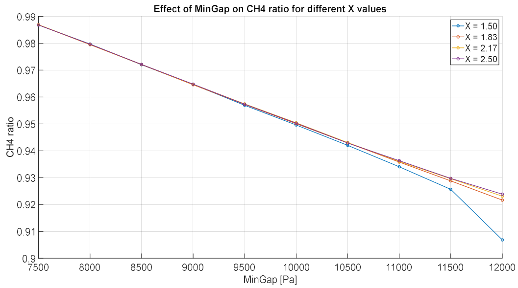
Figure 52 - Diagram showing the trend of the methane concentration as the discharge pressure changes, for different values of X and with a minimum pressure of 5 bar
