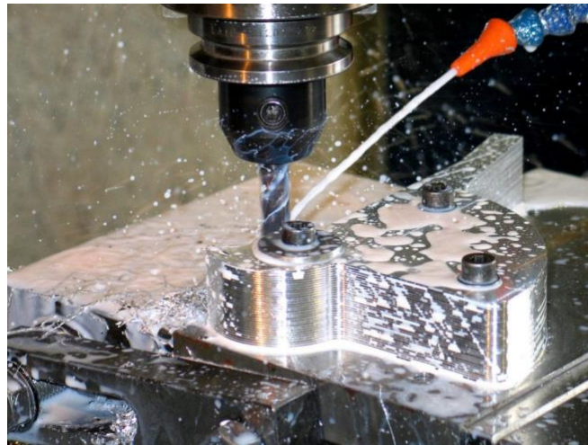
Figure 9 - This image showcases the milling process. The application of a cutting fluid, visible as a spray, serves to cool the tool, reduce friction, and remove chips from the cutting area. [16]
