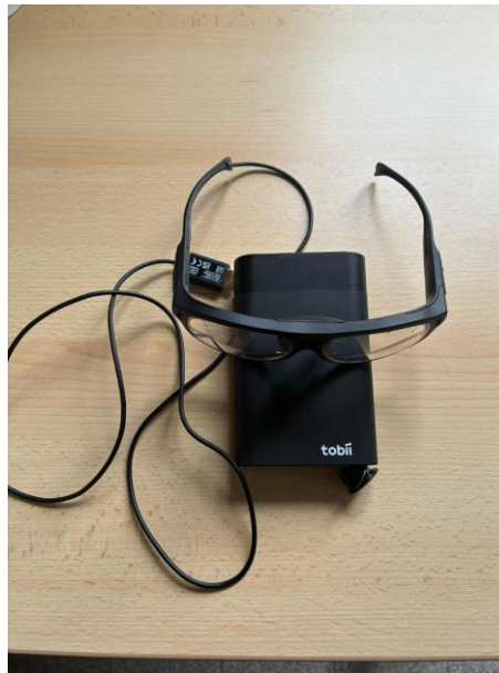
Fig. 2.5 Eye tracker Tobii Pro Glasses 3
