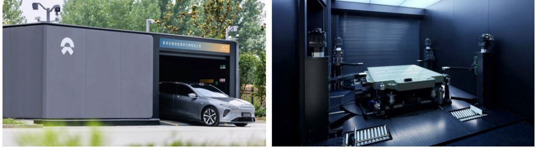
Figure 2.1: NIO Power Swap Station 4.0 (supporting automated battery swap for multiple brands and different vehicle models, i.e. NIO, ONVO and all battery swap strategic partners)
