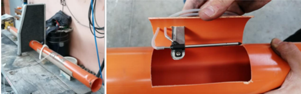
Figure 17: Test rig used for the porosity characterization and detail of the Pitot tube
