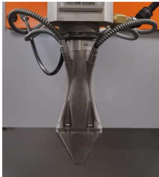
**Figure 1.10:** Deposition head
