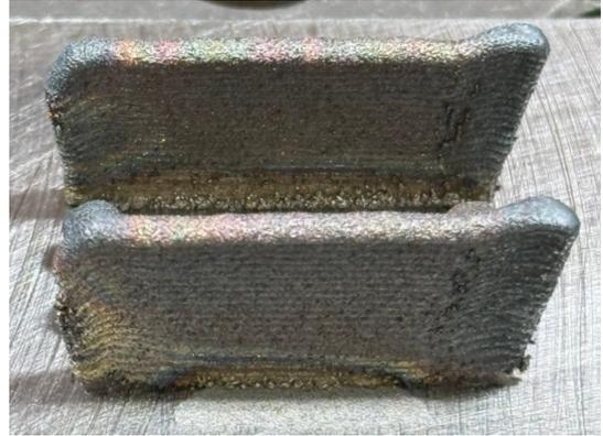
**Figure 3.4:** Deposition test of test geometry 1
