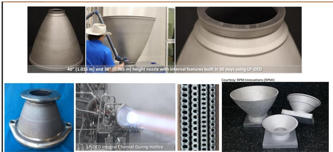
**Figure 1.6:** Large scale manufacturing examples from *"Principles of Directed Energy Deposition for Aerospace Applications"* by NASA, Slide 21
