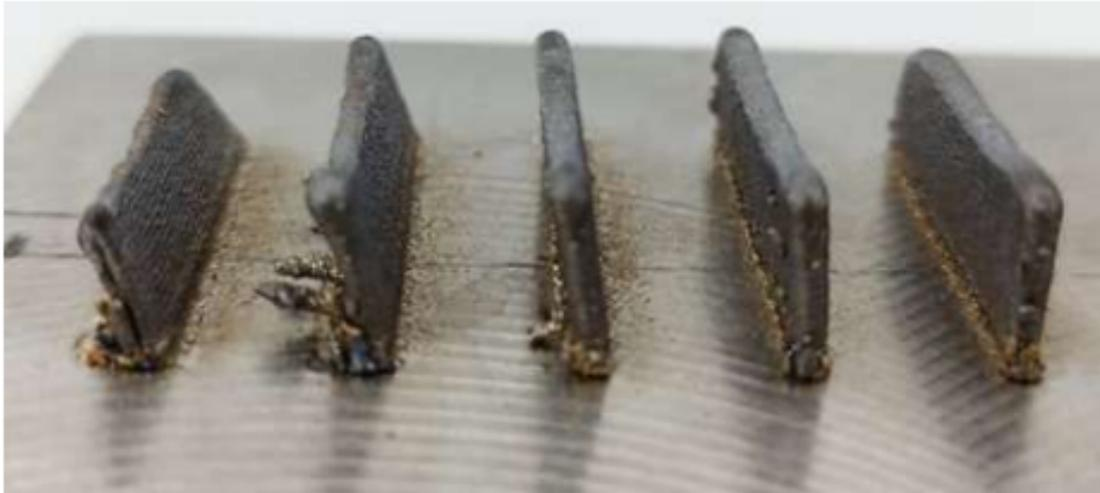
**Figure 2.8:** Overhang effects from  $5^\circ$  to  $25^\circ$
