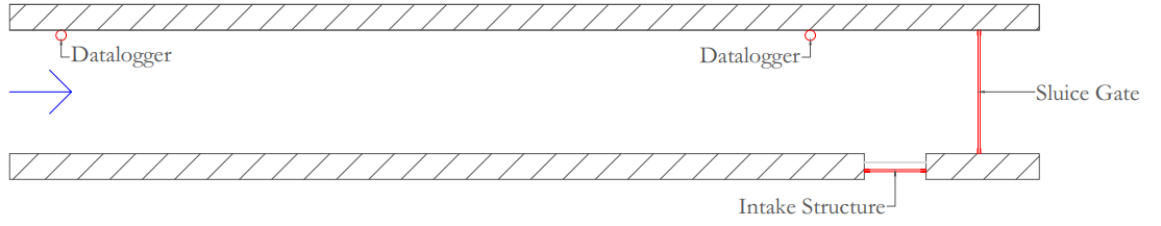
Figure 20. Plan view of the channel showing datalogger arrangement
