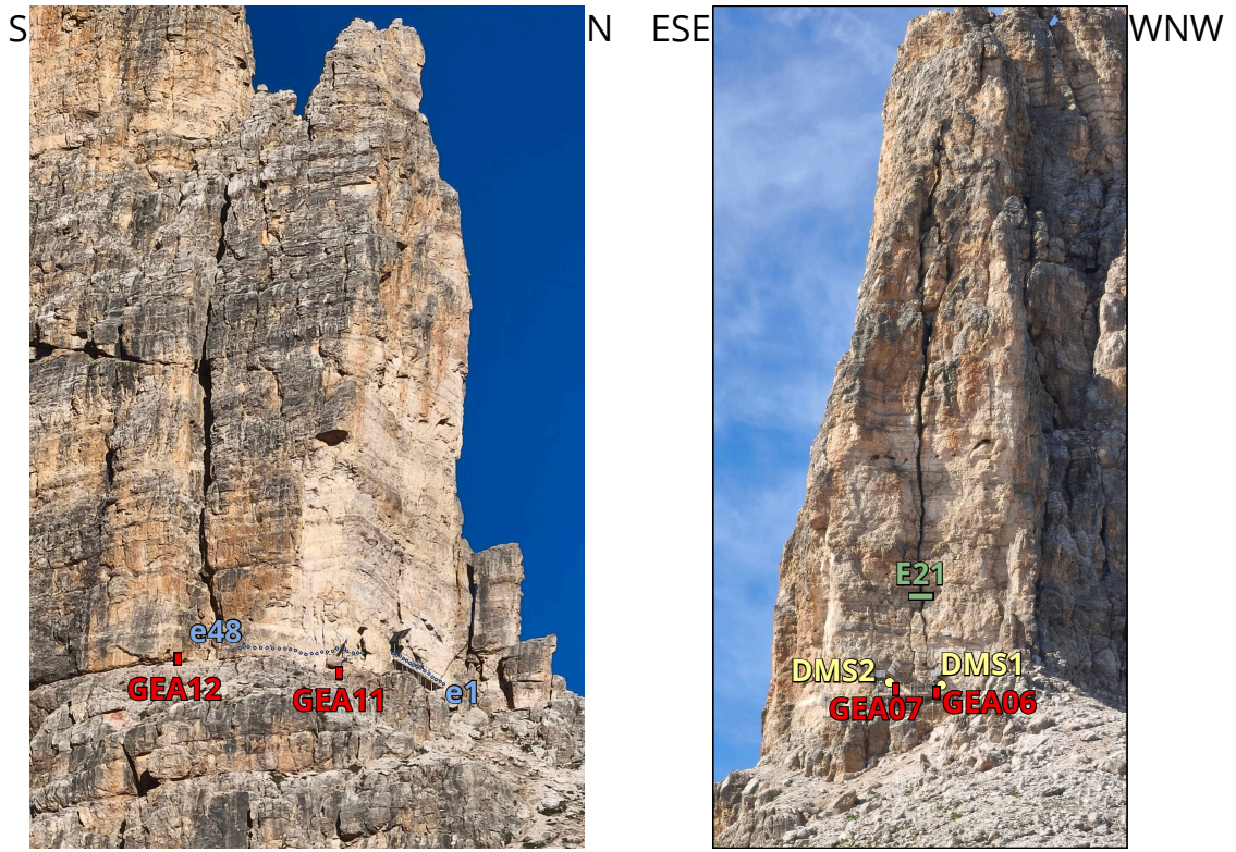
Figure 3.7: Schematic representation of the locations of the instruments within the monitoring site: geophones (GEA06, GEA07, GEA11, GEA12), extensometer (E21), multiparametric columns (DMS1, DMS2) and electrodes (e1-e48).
