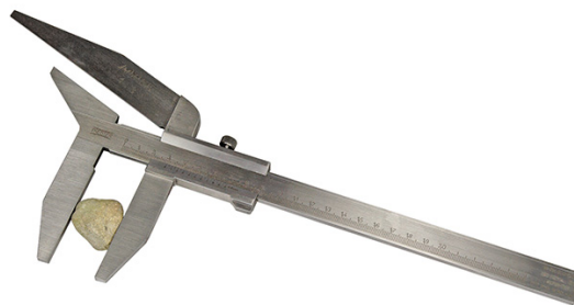
Figure 3.8: Shape index caliper used for measuring the elongation of recycled coarse aggregate particles
