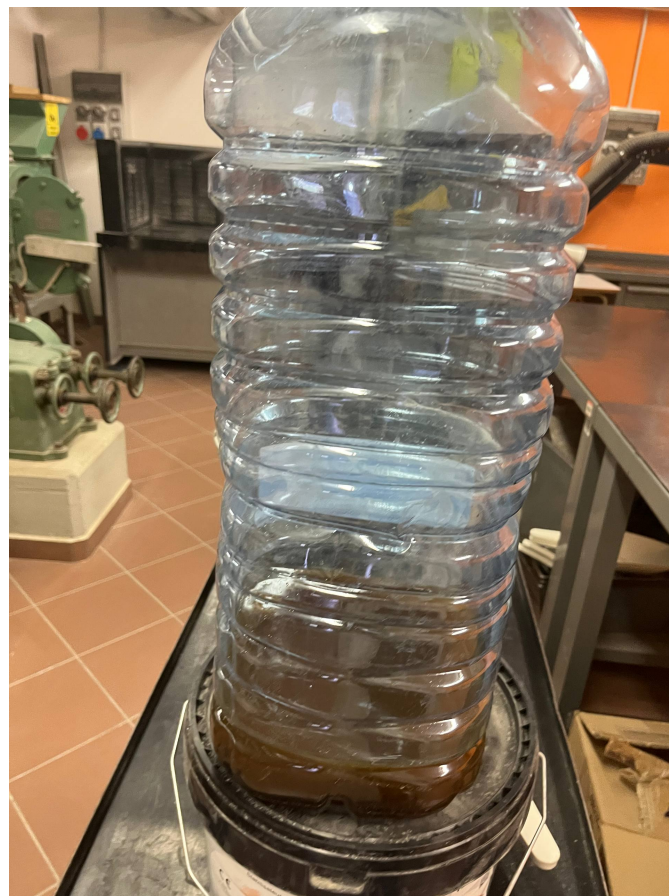
Figure 3.19: Acrylic-based water-reducing admixture (Acrilico Xtend 300R) used in RCA concrete mixes.
