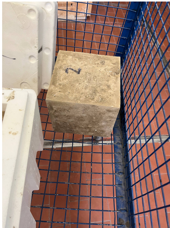
Figure 3.26: Recycled concrete aggregate cube after removal from the mold, prior to curing and compressive strength testing.
