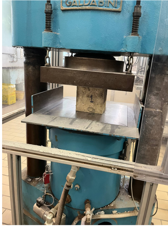
Figure 3.27: Concrete specimen during compressive strength testing.
