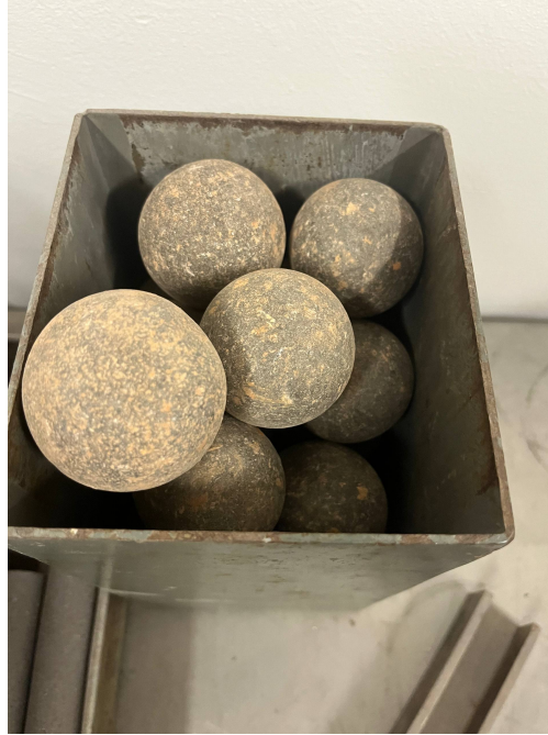
Figure 3.16: Los Angeles Abrasion apparatus used to determine aggregate resistance
