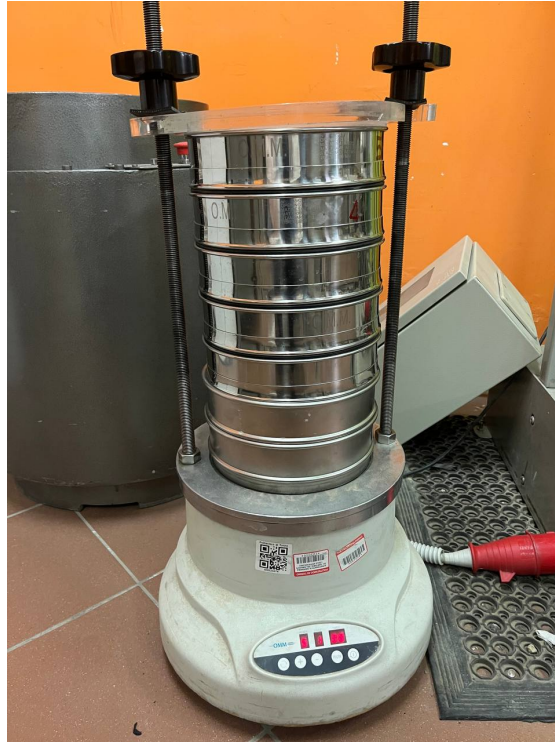
Figure 3.3: Sieving machine used for particle size distribution testing of recycled aggregates
