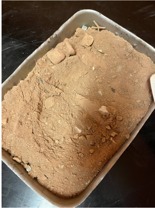
Figure 3.17: Aggregate sample after completion of the Los Angeles Abrasion test.
