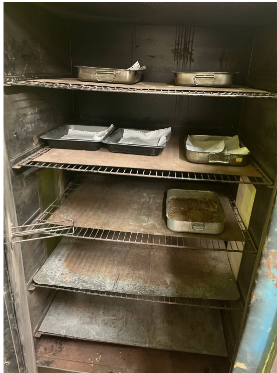
Figure 3.10: Laboratory oven used for drying recycled aggregate samples
