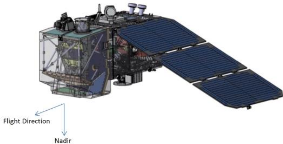
Figure 6 - Schematic view of the deployed Sentinel-2 spacecraft (sources: [14]).
